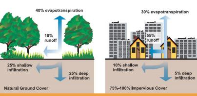
In urbanized areas, greater amounts of impervious cover increase the volume and velocity of stormwater runoff. The Municipal Separate Storm Sewer System (MS4) and flood control channels are designed to convey the runoff to the ocean guickly to protect the community from flooding. Under natural conditions, more stormwater infiltrates into the ground, which provides storage for future use.
