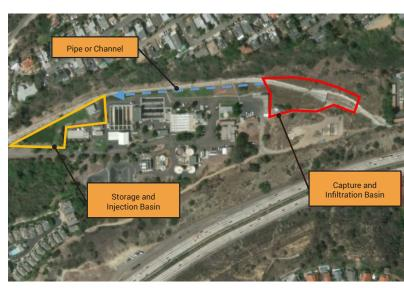
SEWRF Stormwater Capture Elements
